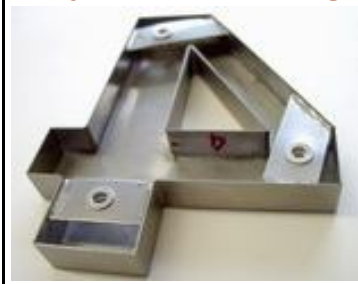
Rear straps with nuts
