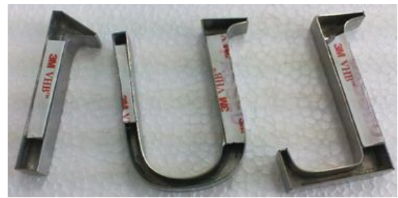
Rear straps with double sided tape
